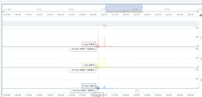
Figure D. Swapping of V and W cells showed that the problem tracked the cell, not the phase.
