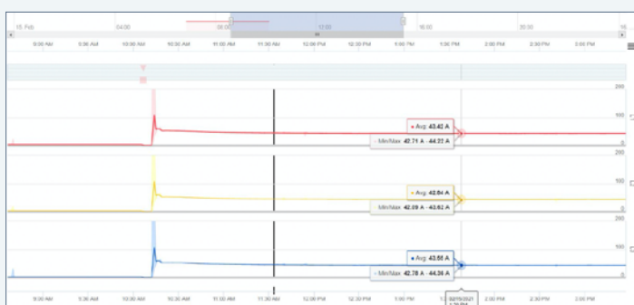
Figure C. Consistent output current when motor was run across the line.
